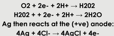
Thus there is a flow of four electrons per molecule of oxygen reduced. This electrical current is directly proportional to the concentration of oxygen in the solution.
